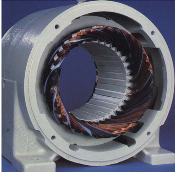
9 - Phase damage, possible voltage unbalance.
