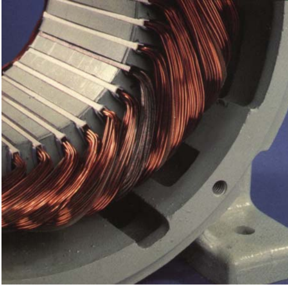
5 - Shorted Coil (sometimes referred to as a 'Hot' coil).
