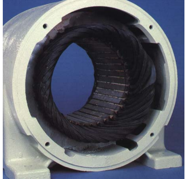
10 - Even burn, loss of cooling, overload, low or high voltage.
