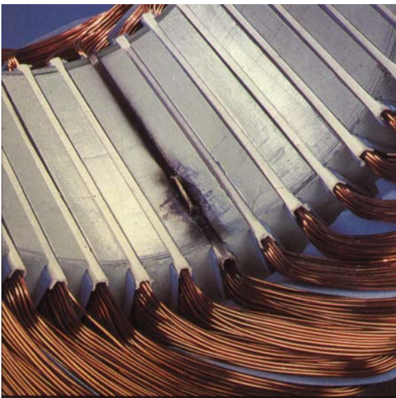
7 - Winding grounded in slot.
