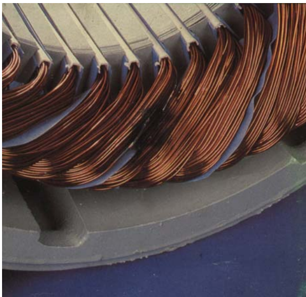
3 - Phase to Phase winding short.
